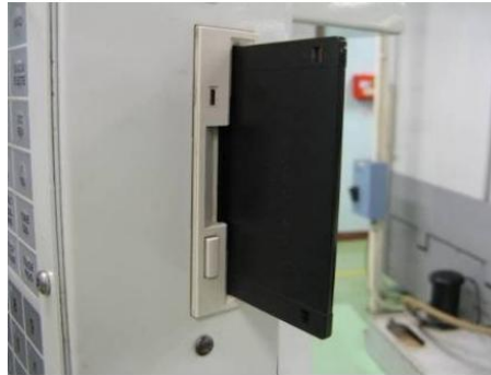
Figure 2.6 Floppy Disk Drive in CNC machine, [16]
