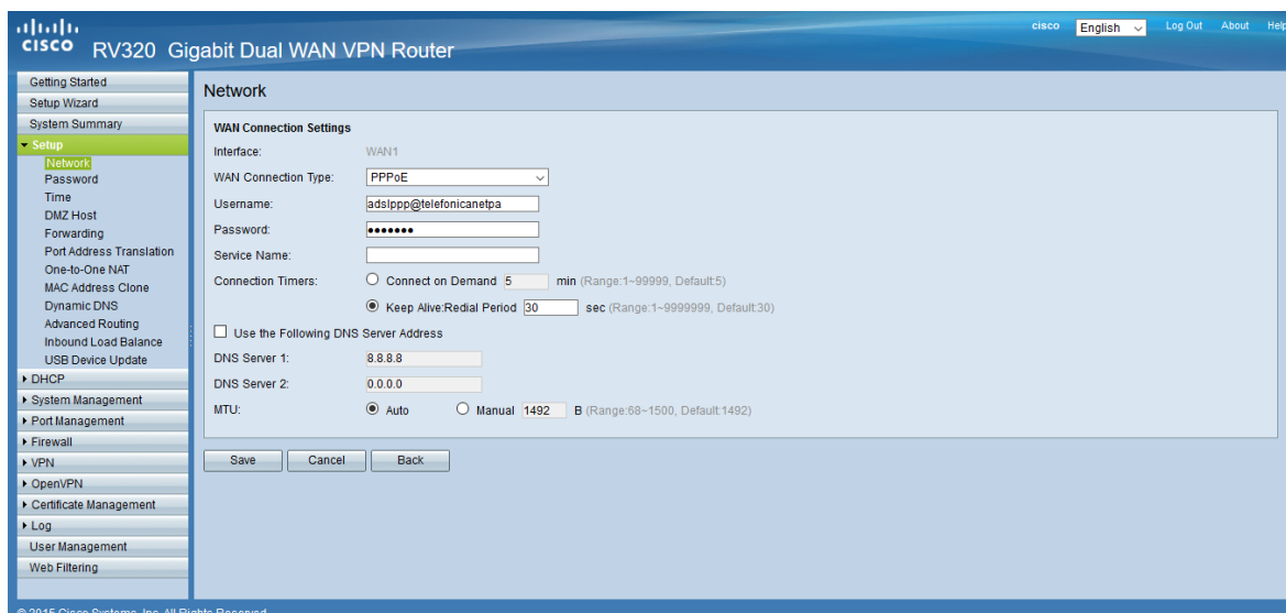
Figure 117. WAN configuration with pppoe
