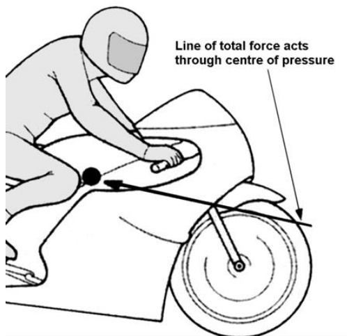
Fig 5.6 In the case shown, the resultant aerodynamic force is acting upward. The horizontal component is the drag force and the vertical component represents a lift force.
