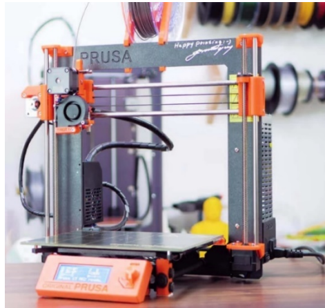
Figura 2-2 Impresora 3D FFF Original Prusa i3 MK2. [6]
