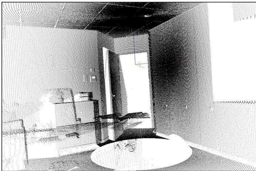
Figure 4: Black & white point cloud from a 3D laser scanner survey [10]
