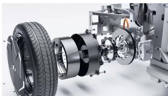
Fig. 72 Motor In-Wheel del Lightyear. (Lightyear, 2022)
