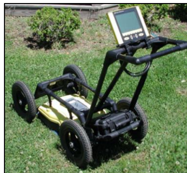
Figure 16 : Ground penetrating radar (GPR) [26]
