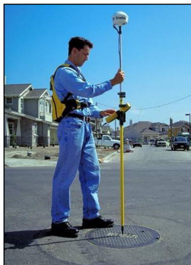
Figure 15 : Sewer system asset mapping [25]
