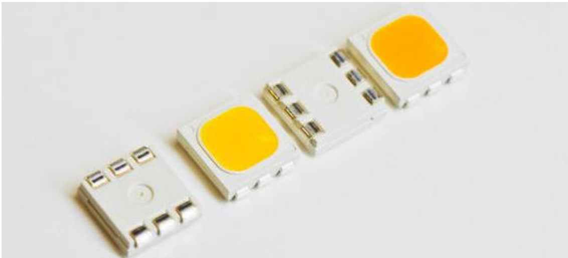
Ilustración 11: LED SMD o Surface Mounted Diode. [5]
