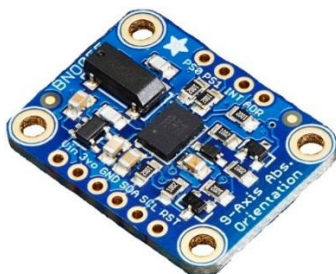
Figura 16: Sensor inercial BNO055
