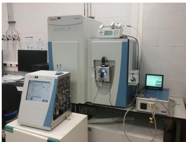
Figura 3.2: Infusión directa-Q-Exactive Orbitrap (ThermoFisher Scientific).
