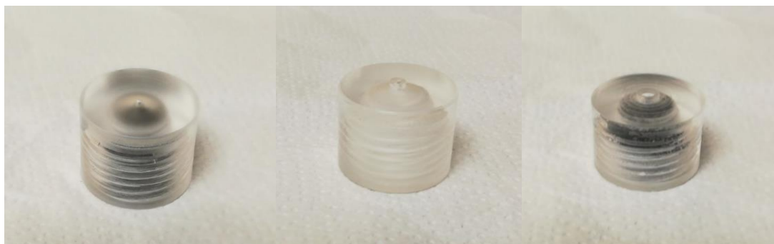
Figura 3. 16 Orificio PMMA, D_i = 1 \text{ mm} ; Tobera PMMA, D_i = 1 \text{ mm} y Tobera PMMA, D_i = 3 \text{ mm}
