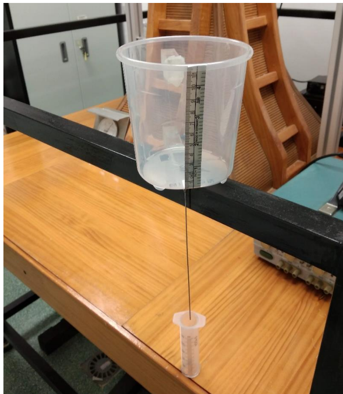
Figure 3.11: Experimental set-up for surface tension assurance based on Tate's law.
