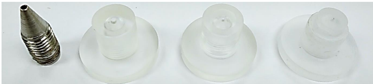
Figure 3.7: Different nozzles used in different experiments, from left to right: 2.35 mm diameter nozzle, 2 mm diameter nozzle, 1 mm orifices for hydrophobic treatment (x 2).
