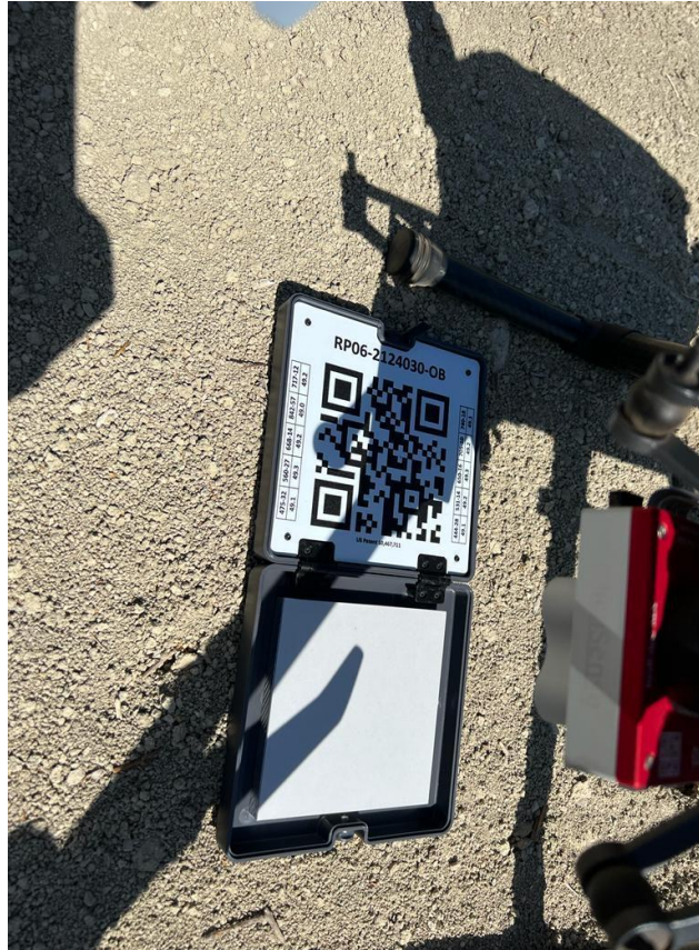
Figure 28: Capture photo of the calibration photo pre-flight
