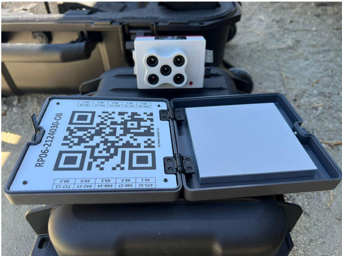
Figure 23: Calibration panel of the multispectral camera
