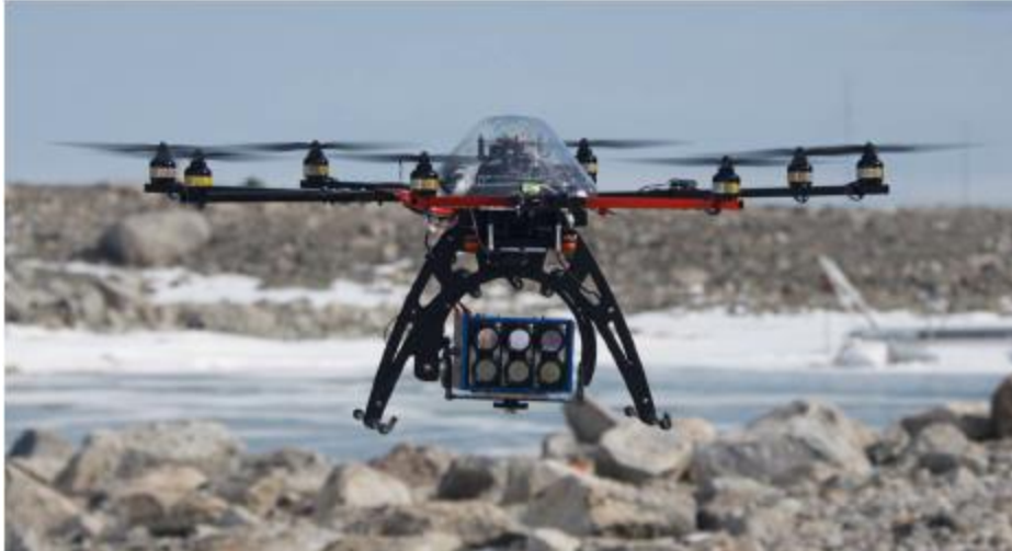
Figure 7: Ortokopter uav fitted with a multispectral camera
