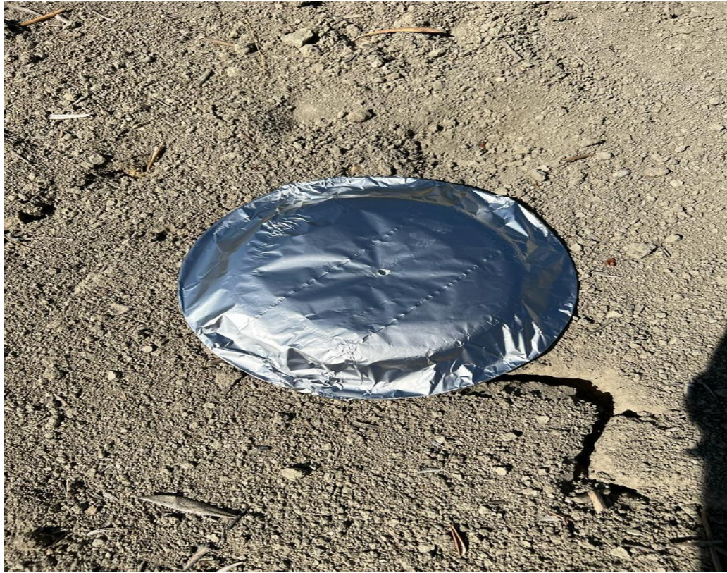
Figure 26: Using a white board as a signalizer for control points
