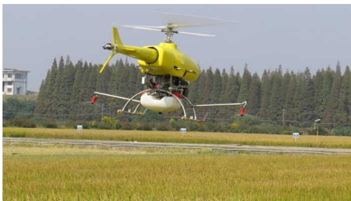
Figura 107. Hércules 30. Agriculture Unmanned Aerial Vehicles (UAV) Sprayers by Homeland Surveillance & Electronics LLC. Dispone de depósito de fitosanitario en su parte inferior (Vehicles)
