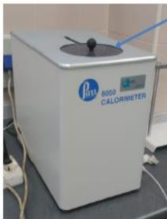
Figure 61: Closing the cover of the calorimetric pump assembly.
