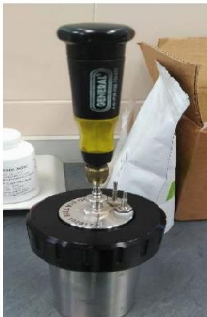
Figure 63: Placement of the tool and removal of the internal pressure.
