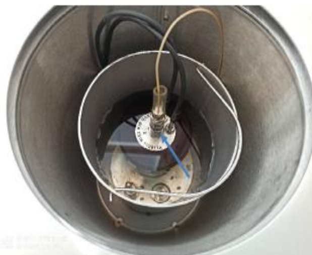
Figure 60: Connection of electrical terminals and the oxygen connector location.
