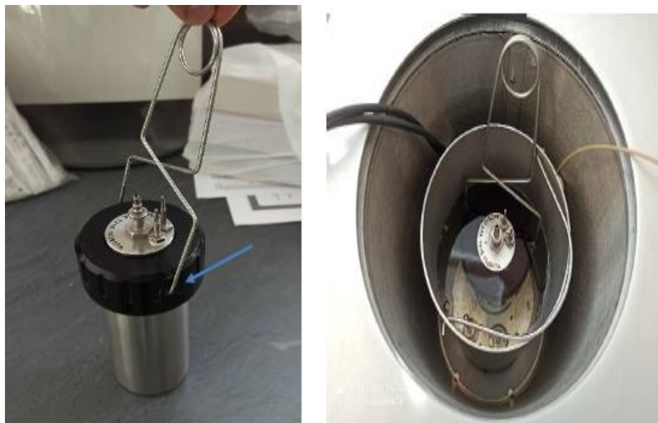
Figure 59: Placement of the support on the screw cap, including the oxygen combustion vessel assembly on the flask.
