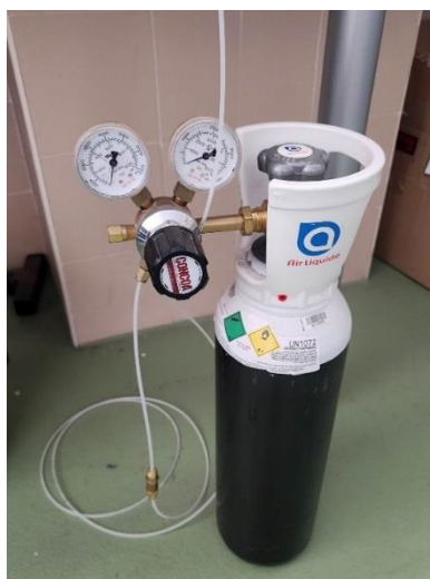
Figure 48: Auxiliary oxygen pressure equipment.
