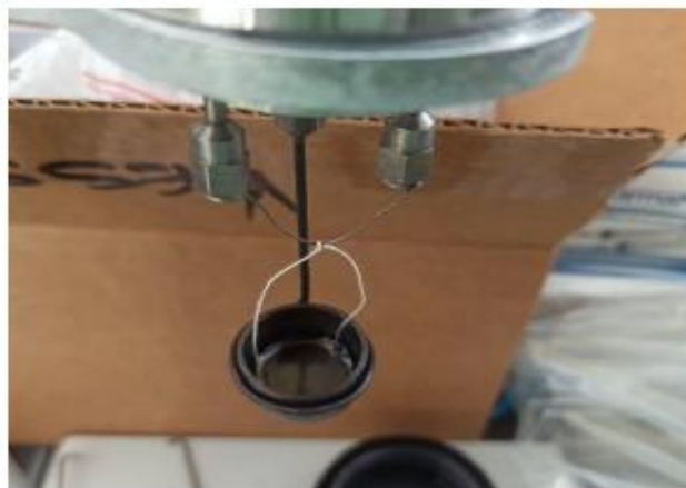
Figure 56: Placement of the cotton thread in the case.
