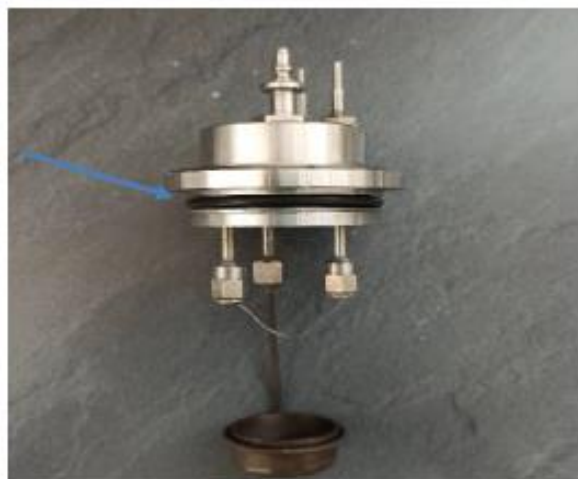
Figure 57: O-ring moistened with distilled water.
