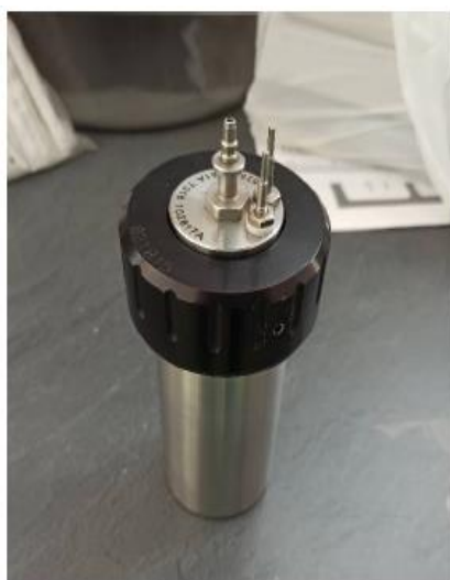
Figure 58: Screwing of the head assembly to the cylinder.
