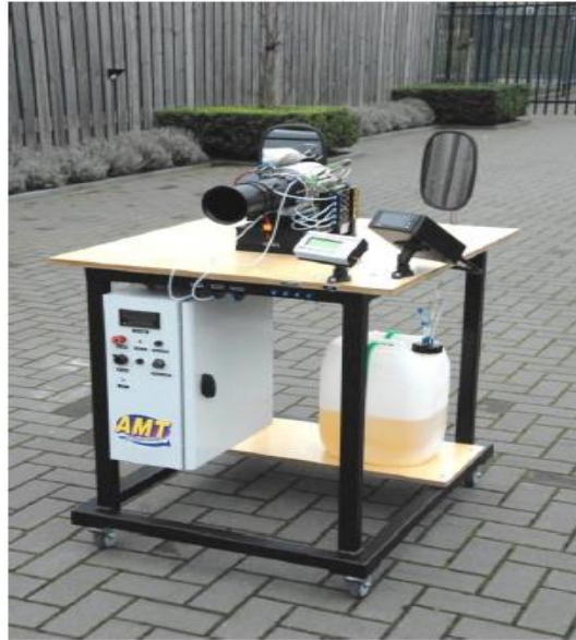
Figure 16: Olympus HP engine in the “university” configuration.
