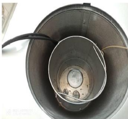
Figure 54: Placing the cuvette in the calorimetric pump assembly.
