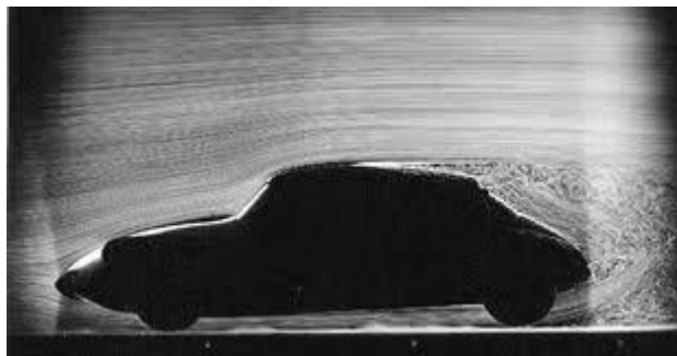
Figure 22 : Flow of air on a car
