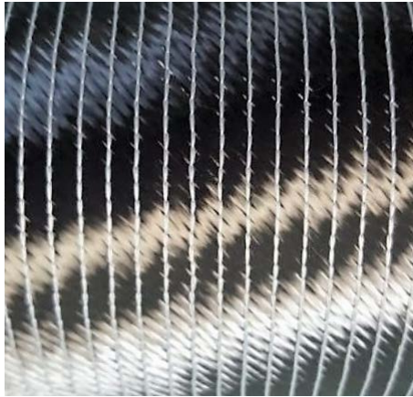
Figura 38. Fibra de carbono triaxial 0/-45/45 450g/m 2 .
