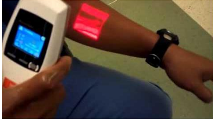
Figura 4.7- Dispositivo Near-infrared vein finder
