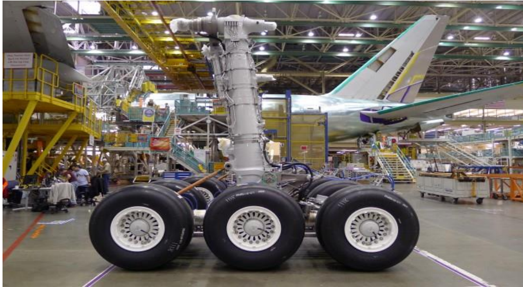
Figure 25: Boeing 777 landing gear
