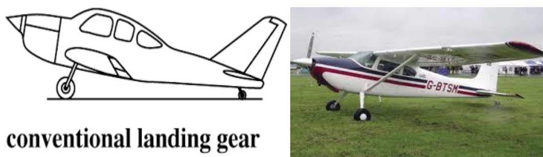
Figure 12: Tail wheel-type Landing Gear
