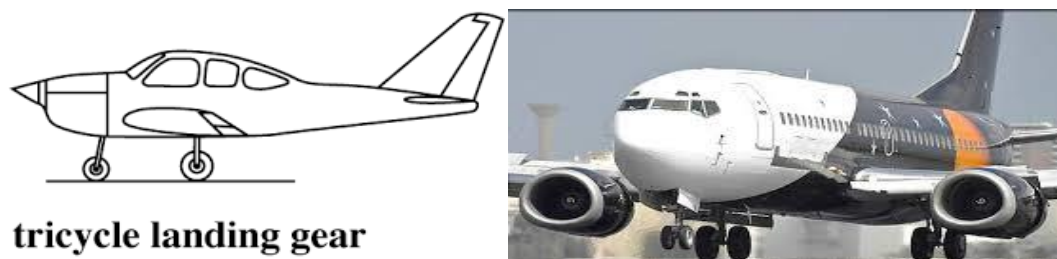
Figure 14: Tri-Cycle Type Landing Gear
