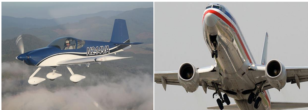
Figure 16: Fixed and Retractable Landing Gear
