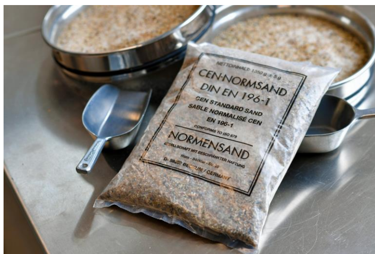
Figura 3.2. Arena normalizada CEN-NORMSAND.
