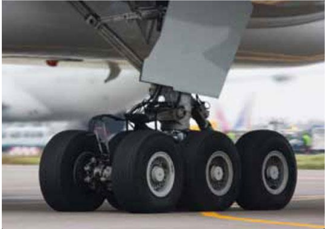
Figure 9: Triple bogie main landing gear assembly
