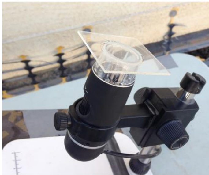
Figura 3.11. Outdoor Soiling Microscope [48].
