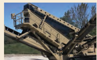
SCREEN 5' x 14' / 1.524m x 4.267m 1000rpm Maximum Optional Ball Deck Available
