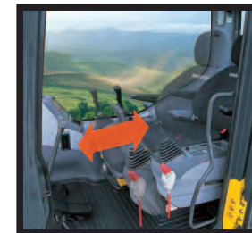
Seat Sliding Amount: 340 mm 13.4", increased 120 mm 4.7"
