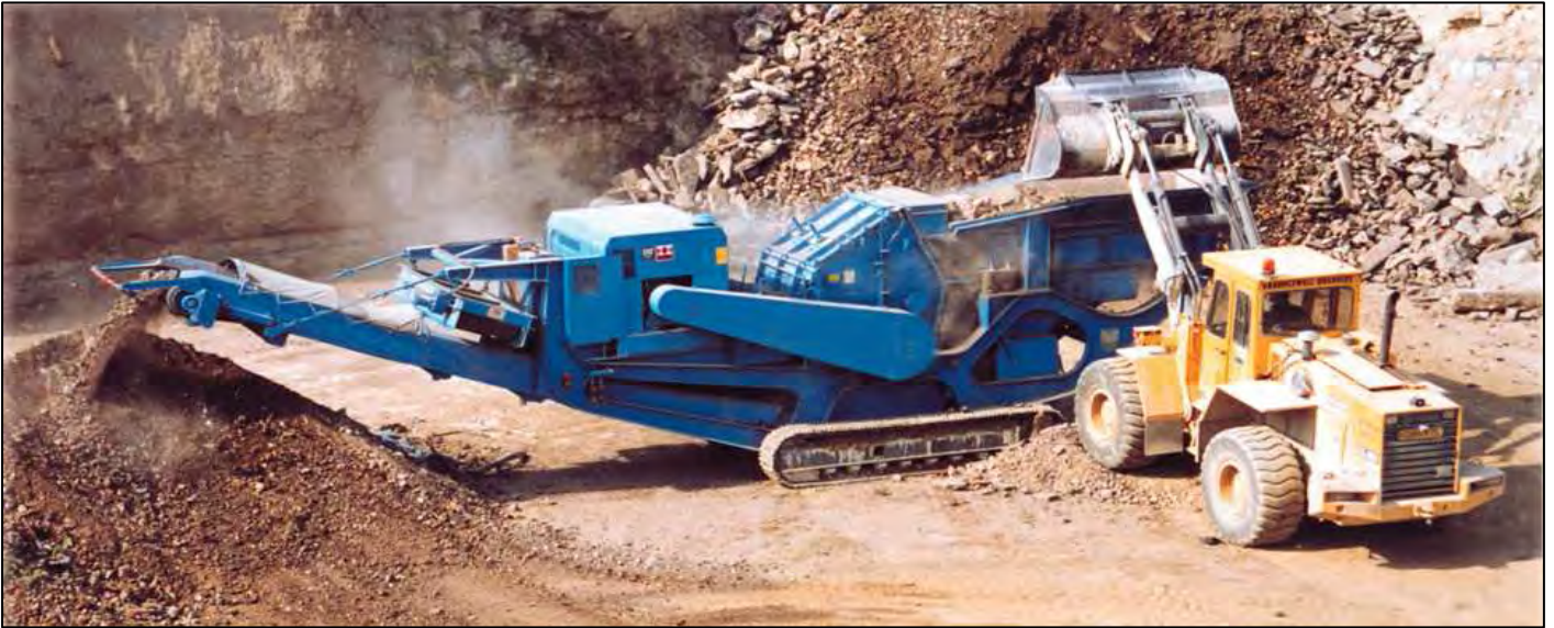
Above photograph features a 428 Trakpactor fitted with the optional side conveyor and magnet
