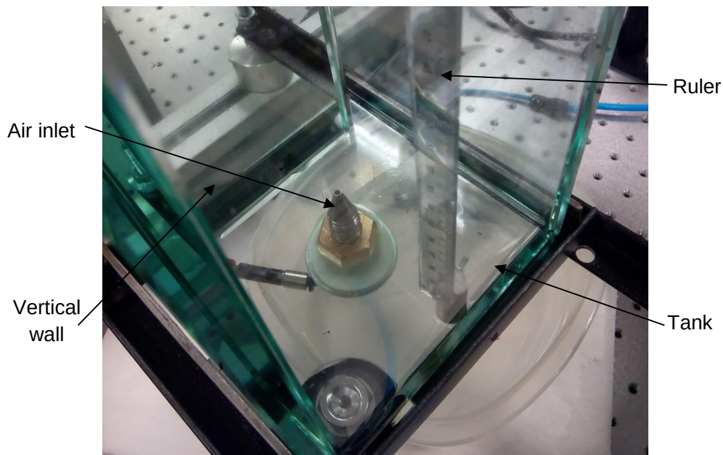
Figure 3.5: Picture of the bottom of the tank, showing all its components and the 2.35 mm nozzle installed.
