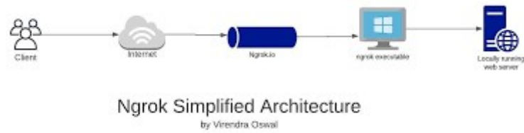
Figure 45. Ngrok simplified architecture
