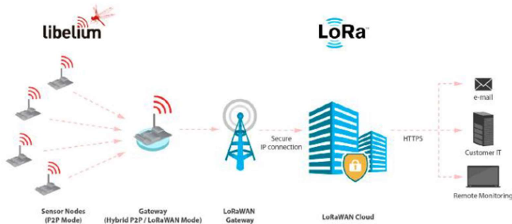
Figure 16. Hybrid mode scheme [18]
