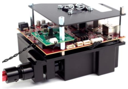
Figura 4.11. Micro NIR de Texas Instruments DLP® NIRscan™ EVM
