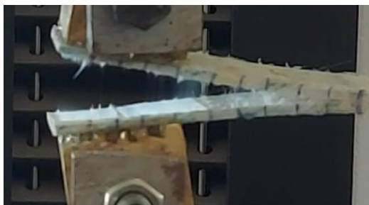
Delamination without bridging
