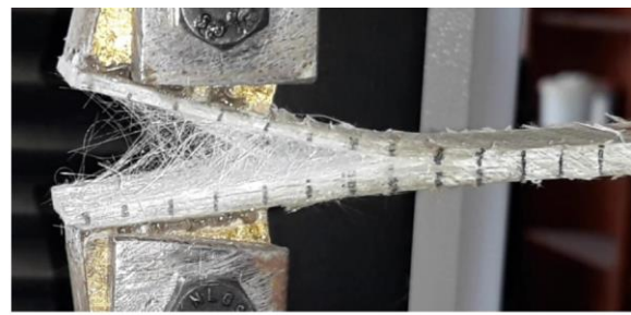
Delamination with bridging
